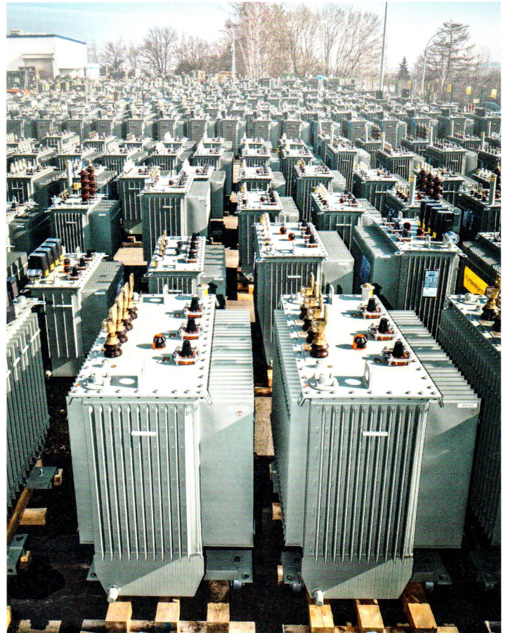
Distribution networks were designed as one-way streets, but they are now characterized by rapid two-way traffic. VRDTs ensure a stable voltage band.
